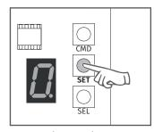
4 • The display will show 0 (disabled), 1 (enable). Use the SEL key to select the desired option and press SET to confirm.
