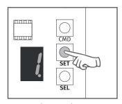
4 • The display will show the value 0 or 1, which identifies the option in which the control board is currently configured. Use the SEL button to put on the desired option. Press the SET button once to save this option.
