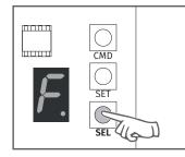
2 • The display will show F. Press the SEL button as many times as necessary until the display shows b.
