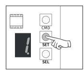
4 • The display will show the value 0 or 4. Use the **SEL** button to put on the desired option. Press the **SET** button once to save this option.
